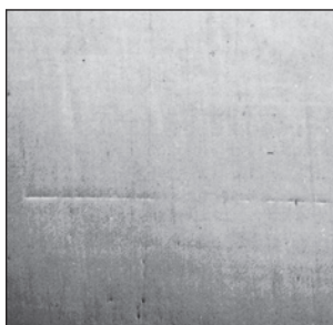
Scratch remains due to overload.
