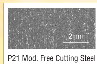
● Comparison of electric discharge machined surface
