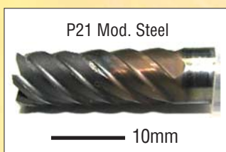
● Comparative example of tool damage in high load conditions of coating carbide end mill
