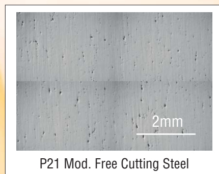
● Differential interference figure comparison of #5000 mirror polished surface (2×2 sequential photographs)
