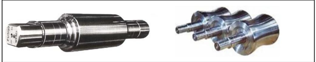
**H**igh chromium steel rolls have a low carbon content (0.8-1.5%) and are composed of a bainite matrix with a small amount of chromium carbide in the structure. The bainite matrix is made by a special heat treatment procedure, making the hardness and tensile strength of chromium steel rolls higher than that of other low alloy rolls such as adamite. Chromium carbide is higher in hardness than ferrous carbide. Therefore, these rolls perform better than low alloy rolls.
