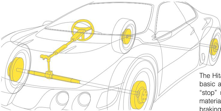
The Hitachi Metals Group supports the development of basic automotive functions, that is, “drive,” “turn” and “stop” motions, by supplying parts, components and materials for the electric power steering and antilock braking systems.
