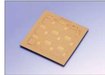
LTCC substrates used in electrical equipment
