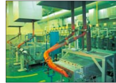
Combustion testing of an exhaust manifold via an exhaust gas simulator
