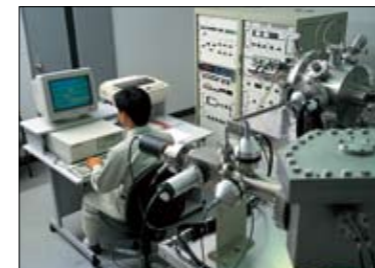
Microelement survey of materials using a GD-MS (Glow discharge mass spectrometer)
