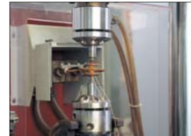
Thermal fatigue test to analyze heat resistance properties of a new material
